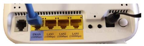
3. The blue lead then connects into the IDU's (Black box labelled Alvarion) Ethernet port (On the side)
