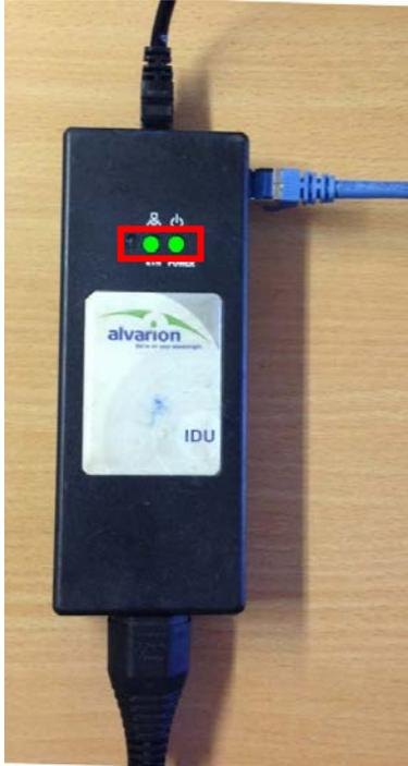
The **black Ethernet** cable goes off to the aerial and must be in the 'Radio' port in the end of the power supply, this is placed at the top. The **power cable** is connected at the bottom and the **blue cable** plugs into the 'Ethernet' port on the Radio's power supply, this is placed at the side.
