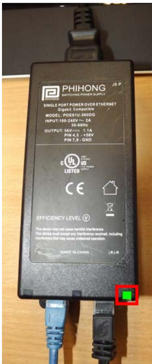
The **black lead** at the bottom right goes off to the aerial and must be in the 'out' port in the end of the Radio power supply, this is placed at the bottom of the power supply. The **blue cable** connects to the 'in' port and the **power cable** is connected at the top of the power supply.
