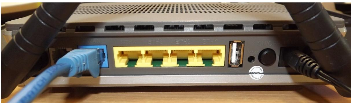
3) The **blue** lead then connects into the Radio's power supply (Also known as an IDU).
